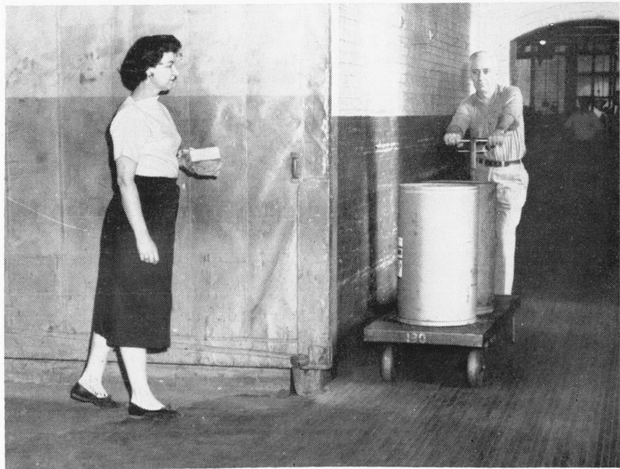
James Dugan, of Mfg. Trucking, demonstrates how an accident could happen when a skid of work being moved with a hand jack is pushed instead of pulled along. Pauline Semplenski (Closing Room) poses as the possible victim.
